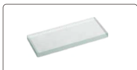
50mm reading scale (check magnification accuracy)
