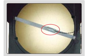
edge detector (for ISP-A6000E)
